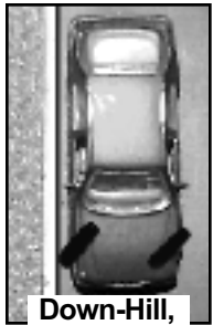
Down-Hill, with curb.
