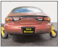
There is no better way to learn the power of the Ten Zone Control Habits than to drive the SkidMonster. It is a specially equipped car that recreates, in a safe training environment, the effects of lost of traction. It trains drivers in use of vision to control the vehicle.
