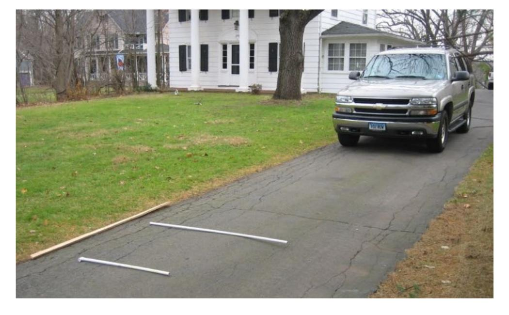
Here, the length of wood is aligned with the SUV's right side limitation. The two white pipes represents the nearest point of pavement seen by a driver seated high and one seated lower.
