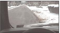
The skid continues to develop. The actions to take are no pedals and fully steer left to get back on target.
